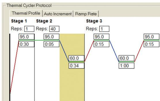
Figure 1. Shuttle PCR standard protocol
