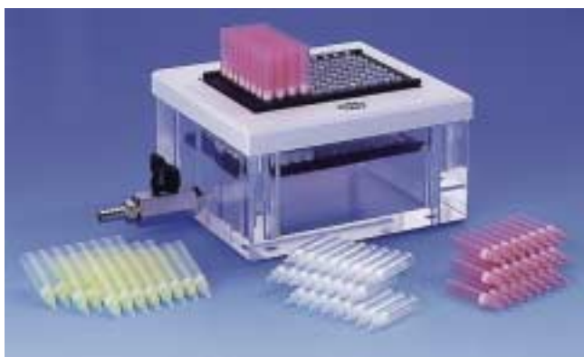
Figure 1. The NucleoVac™ vacuum manifold. This high-quality acrylic manifold is easy to operate and maintain. It holds 12 Multi-8 strips at a time and can also accommodate individual NucleoSpin columns. NucleoSpin Multi-8 Plus Filter Strips (pink; on top of manifold) filter the bacterial lysate and deliver the cleared suspension containing plasmid DNA into NucleoSpin Multi-8 Strips (white; inside manifold) for further processing. The NucleoVac manifold is sold separately.
