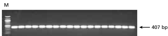
Figure 2. The BD Sprint™ TITANIUM™ Taq 384 Plate produces consistent high-throughput PCR results. Each well was reconstituted with 10 \mu l of Milli-Q water containing 20 ng of Control Calf Thymus DNA and 10 \mu M of primers specific for a 407-bp segment of the bovine pancreatic trypsin inhibitor (BPTI) gene. PCR was carried out under the following conditions: 95°C for 1 min, followed by 30 cycles of 95°C for 15 sec and 68°C for 30 sec, then 68°C for a final 3 min. 5 \mu l of each PCR reaction was electrophoresed on a 1.2% agarose/TAE gel. Lane M: 100-bp DNA size marker.
