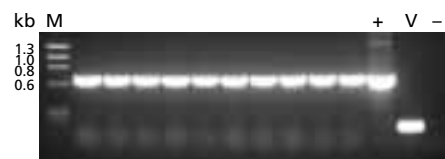
Figure 2. The BD Creator™ Cloning System generates a high frequency of recombinant adenoviral constructs. An expression cassette was transferred into the BD Adeno-X™ LP Promoterless Expression Vector using Cre recombinase. Recombinant adenoviral DNA was amplified in E. coli GC10. Following selection, 10 colonies were picked at random and analyzed by PCR using vector specific primers and the BD Sprint™ TITANIUM™ Taq 384 Plate (#K1952-1 or #639552). 10 colonies tested positive for the presence of a DNA insert. A total of 36 experiments using 13 different genes and any one of the three expression systems generated a cloning efficiency of 87.7% (data not shown). +: positive control. V: vector only. -: negative control. M: \lambda Hind III and \phi X174/Hae III.
